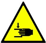
RISK OF CRUSHING - Lifting or lowering the tray, can jam and crush limbs.
