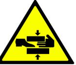
MAINTAIN A 25mm DEGREE ABOVE THE SEAT OBJECTS ON THE DESK WHEN THE DESK IS AT MAXIMUM HEIGHT, AND BETWEEN THE DESK AND ADJACENT OBJECTS. - Position the desk, accessories and surrounding objects to allow full range of work surface motion, without risk of rope pulling, limb jamming or collision with other objects (shelves, electrical outlets and wires, door handles, window sills, cabinets, etc.).
